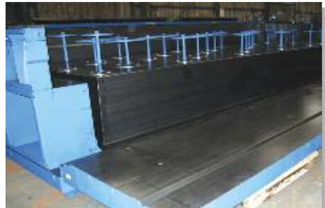
Sideforms pivot open for stripping.
