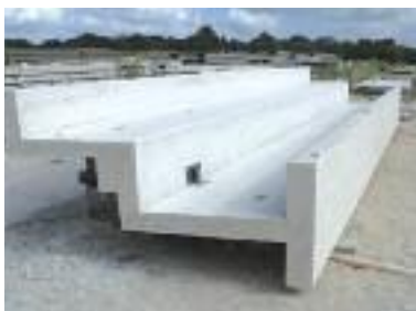
Some risers called for a broom finish with a sand blasted vertical face and were poured in 3 stages with no cold joints. Lower sections were allowed to initial set before the broom finish was added. A second pour filled the top section. Finally, the vertical face that required sand blasting was poured with a dryer mix.
