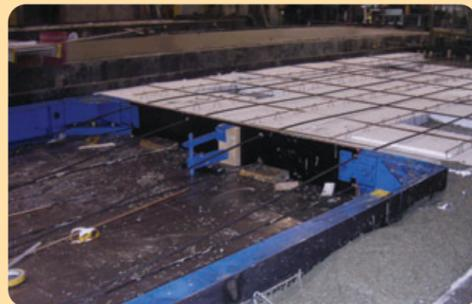
Magnetic corner system used as a door block-out with steel side sections and wood at the top and bottom held in place with an outrigger magnet.
