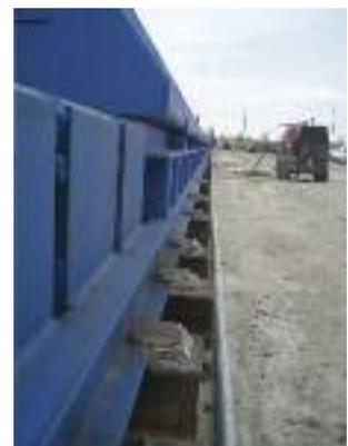
St. Louis Prestress recently installed a 320-foot Box Beam bed. This photo is a good example of how a self-stressing form should be clipped down, with welds on the side of the shims as well as the toe to constrain the form laterally, while permitting longitudinal shortening when the bed is stressed.
