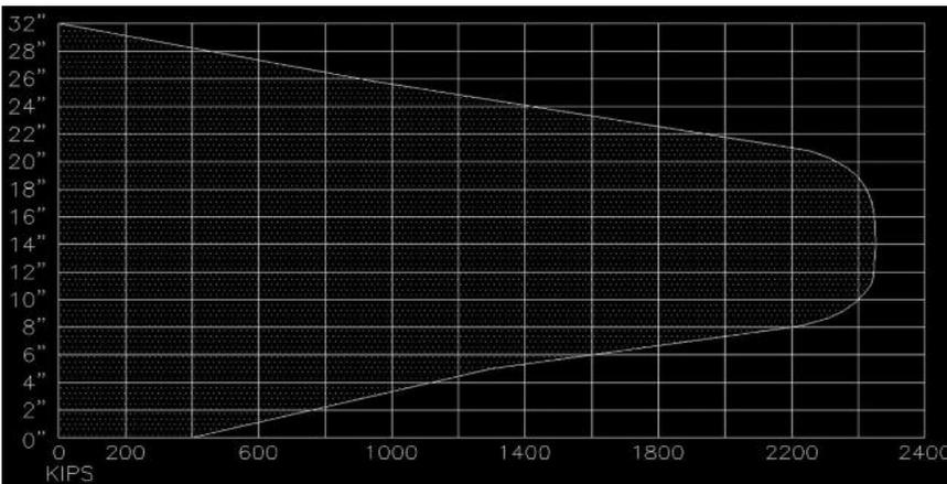
Stress envelope for NEXT Beam form, designed for double row of 0.6 strand and 2400 maximum kips.
