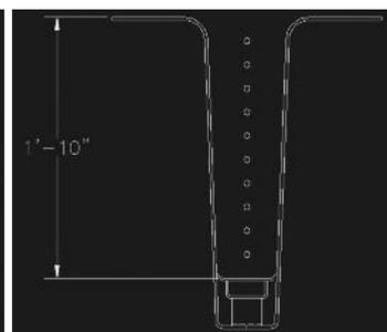
**3.** Adding 4" stem fillers moves the C.G. to 15" with 10 strand @ 30 kips each. Total capacity still falls within the stressing envelope.
