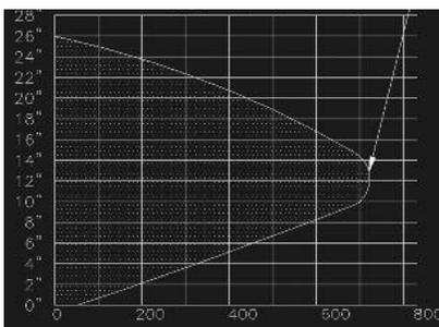
**1.** Typical stress envelope for a double tee with 2'-2" stems designed for a single row of 1/2" strand for a total capacity of 720 kips.
