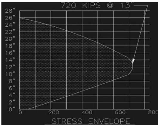
Stress envelope for form designed for 1/2" strand and 720 maximum kips. A change to 0.6" strand will definitely overload the form.
