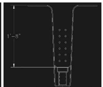
**4.** Double row of strand with 6" filler. Each stem has 12 strand @ 30 kips @ 13" C.G. Total kips does not exceed the capacity of the form, but the position of the strand will locally overload the form.
