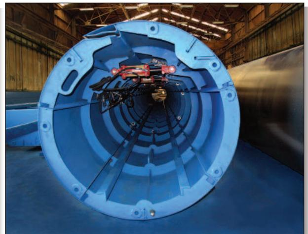
42" hydraulically actuated, collapsible void
